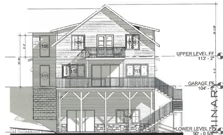
1 SOUTH BUILDING ELEVATION A5.0 SCALE: 1/8" = 1'-0"
