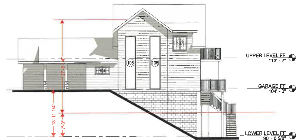
3 WEST BUILDING ELEVATION A5.0 SCALE: 1/8" = 1'-0"
